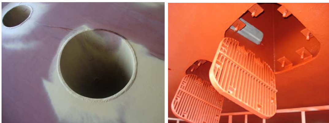
(6) Plating of sea chests. Also side shell plating in way of overboard discharges, as considered necessary by the Surveyor.
