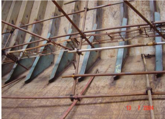
Above and to the left – Typical defect, wastage of cargo hold side shell frames of single skin bulk carriers
