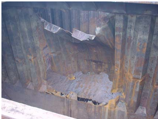
Images depicting a failed transverse bulkhead and a typical corrugated bulkhead reinforcement following a URS 19 assessment
