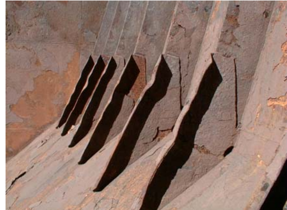
Above and to the left – Typical defect, wastage of cargo hold side shell frames of single skin bulk carriers
