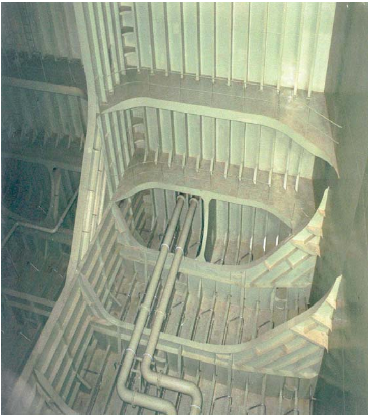
FAIR - Condition with local breakdown of coating at edges of stiffeners and weld connections and/or light rusting over 20 per cent or more of areas under consideration, but less than as defined for poor
