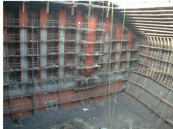
Images depicting a failed transverse bulkhead and a typical corrugated bulkhead reinforcement following a URS 19 assessment
