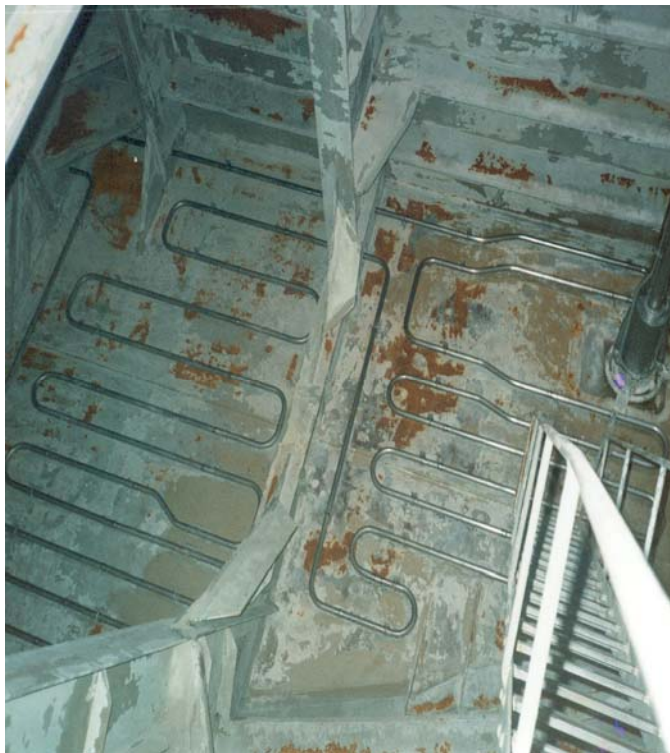
FAIR - Condition with local breakdown of coating at edges of stiffeners and weld connections and/or light rusting over 20 per cent or more of areas under consideration, but less than as defined for poor
